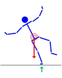
when forces or disturbing moment is applied on a body such that on removal of that force or moment the original position is never restored but rather continually moves to new positions is called unstable equilibrium.
