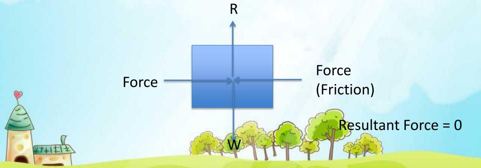
Equilibrium of a body is defined as the state when all the forces and actions acting on the body nullify each other resulting in a stable, balanced and unchanging position.
